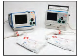
OneStep Electrode Pads are compatible with ZOLL® R Series® and M Series® defibrillators.
