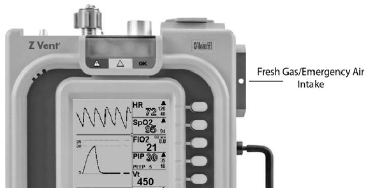
Figure 3-3 Fresh Gas/Emergency Air Intake
