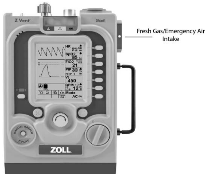
Figure 2-4 Fresh Gas/Emergency Air Intake
