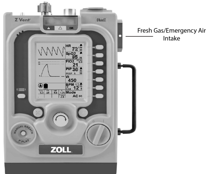
Figure 2-4 Fresh Gas/Emergency Air Intake
