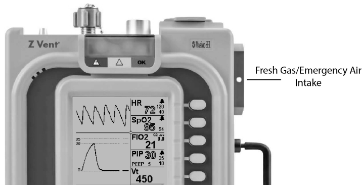
Figure 3-3 Fresh Gas/Emergency Air Intake
