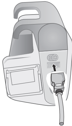
Figure 10-3 Connecting the SpO 2 Sensor to the X Series Advanced Unit
