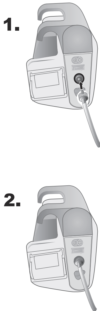
Figure 8-1 Attaching a Dual Lumen Hose to the X Series Advanced Unit
