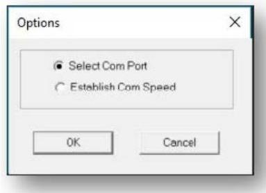
Select the communications port that the PC will be using to transfer data to or from the AED. If using a USB-Com adapter, select the check box More Com Ports for Com Port options Com5 through Com8. Click OK to return to the MDLink window.
