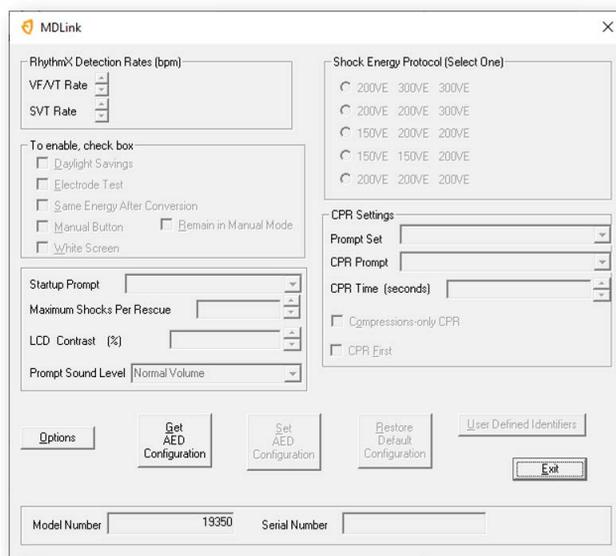
After MDLink successfully retrieves the parameters, click OK to return to the MDLink window. Set AED Configuration, Restore Default Configuration and User Defined Identifiers buttons will be enabled.
